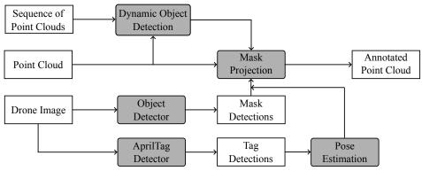
Figure 11: Annotation process of the proposed dataset. Object detections from the drone's image are projected onto the point cloud using the drone's pose determined from AprilTags on each acquisition unit. The projections are further refined using dynamic objects detected within the entire acquisition sequence.
