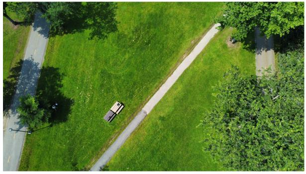
Figure 10: Example of an aerial image taken from a drone. Picture taken from a DJI Mini 2 drone flying at an altitude of 50 m above the Grand Axe on Laval University's campus. The bicycle lanes visible on both sides of the images are approximately 50 m apart. The AprilTag on the picnic table is detectable from this picture and will be made bigger for the data collection process.
