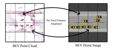
Figure 14: Integration of the JEPA framework with the BEVOcc dataset. The point cloud encoder generates feature embeddings  $(s_x)$  from the point cloud input. Simultaneously, the BEV encoder produces feature embeddings  $(s_y)$  from the aerial image input. The network is trained to predict  $s_y$  from  $s_x$ , effectively learning features within the point cloud that are compatible with the BEV perspective of the same scene.
