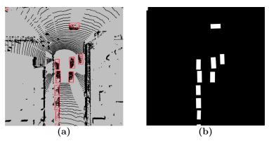
**Figure 5: Mask generation from bounding box labels.** (a) Point cloud from Waymo Open Dataset [76] with bounding boxes drawn around cars. (b) Resulting masks generated from the bounding boxes in (a) Each instance corresponds to a distinct mask, shown here in one image for simplicity.
