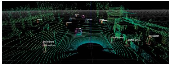
**Figure 2: Illustration of an object detection task.** The primary goal of object detection is to accurately locate and classify objects (e.g., vehicles, pedestrians, and cyclists) within a 3D point cloud. We show here detected objects with bounding boxes and labels with their respective class names. Image created using data from Déziel *et al.* [6].
