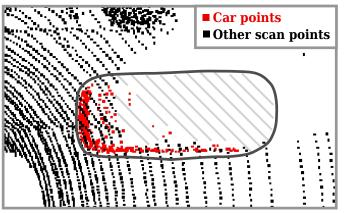
Figure 1: Example of self-occlusion in SemanticKITTI[5] from a BEV perspective. The red points denote a car instance, with its complete footprint outlined in grey. The side of the car facing the LiDAR sensor hides the remainder of the object, resulting in an absence of points on the rest of the object and behind it.
